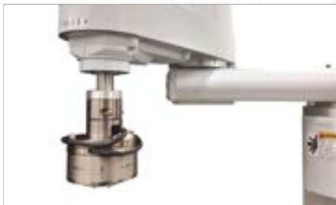
Epson force sensors offer both high sensitivity and high rigidity, allowing for successful high-precision applications when teaching or vision are not enough
