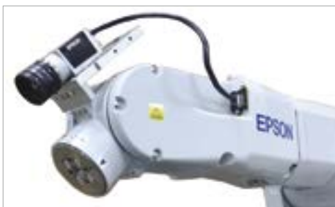
Epson 6-Axis robots work with fixed or mobile-mounted cameras
