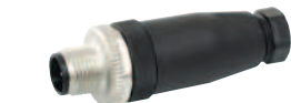
MALE M12, 4-pole, SCREW TERMINAL Operating Voltage: max. 250V AC/DC Connection Diameter: max. .75mm 2 Cable Diameter: 4-6mm Art. Number: 7000-12701-0000000
