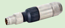
MALE M8, 4-pole, IDC Operating Voltage: max. 32V AC/DC Connection Diameter: .25 - .5mm 2 Cable Diameter: 4-5.1mm Art. Number: 7000-08341-0000000
