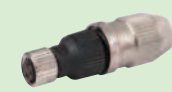
FEMALE M8, 3-pole, IDC Operating Voltage: max. 32V AC/DC Connection Diameter: .25 - .5mm 2 Cable Diameter: 4-5.1mm Art. Number: 7000-08361-0000000
