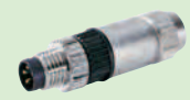
MALE M8, 3-pole, IDC Operating Voltage: max. 32V AC/DC Connection Diameter: .14 - .34mm 2 Cable Diameter: 2.5-5.1mm Art. Number: 7000-08331-0000000
