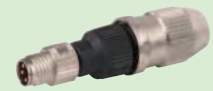
MALE M8, 3-pole, IDC Operating Voltage: max. 32V AC/DC Connection Diameter: .25 - .5mm 2 Cable Diameter: 4-5.1mm Art. Number: 7000-08321-0000000
