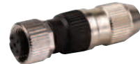
FEMALE M12, 4-pole, IDC Operating Voltage: max. 32V AC/DC Connection Diameter: .25 - .5mm 2 Cable Diameter: 4-5.1mm Art. Number: 7000-12601-0000000
